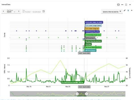
Interval data viewer showing meter interval, register and event data all on the same timeline.
